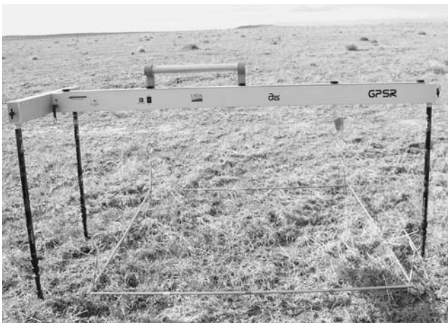
Figure 2. Photograph of the fully assembled laser point frame used to measure cover on a shortgrass prairie.
