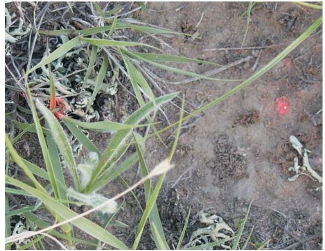
Figure 3. Laser point or dot on vegetation and bare ground. Note halo and center of dot.
